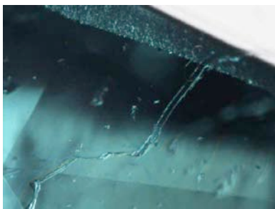
Figure 1a: An example of faceted emerald held in one piece only by a wide tract of hardened resin.
